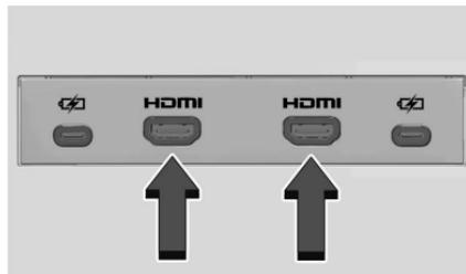
The HDMI input allows an HDMI A/V cable to be connected from an auxiliary device such as a camcorder, video game system, or Apple device. A cable from Apple is required for Apple devices.
