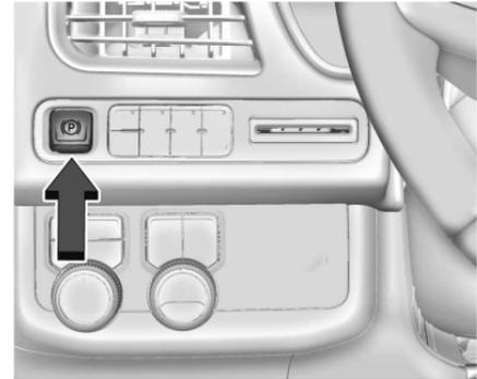
The Electric Parking Brake (EPB) can be applied when the vehicle is off. If there is not enough electrical power, the EPB cannot be applied or released. To prevent draining the battery, avoid unnecessary repeated cycles of the EPB.
