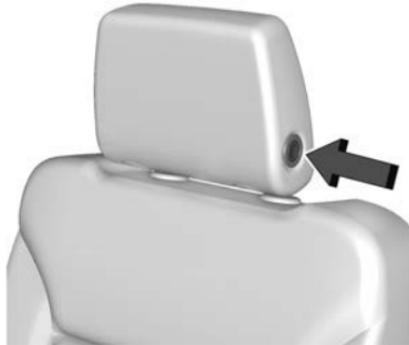
To fold the head restraint, press the button on the side of the head restraint.
