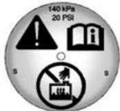
1. Remove the coolant surge tank pressure cap when the cooling system, including the coolant surge tank pressure cap and upper radiator hose, is no longer hot. Turn the pressure cap slowly counterclockwise about one full turn. If a hiss is heard, wait for that to stop. A hiss means there is still some pressure left.
