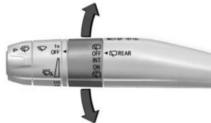
The rear window wiper/washer controls are on the end of the turn signal/windshield wiper lever.
