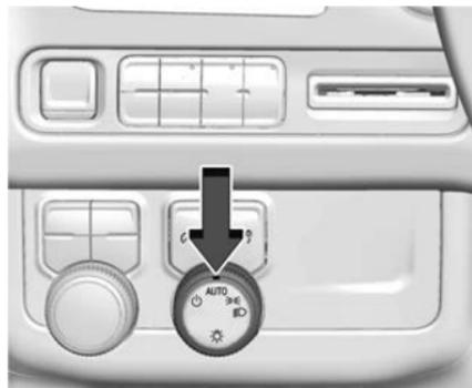
The exterior lamp control is on the instrument panel to the left of the steering wheel.
