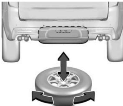
7. Make sure the tire is stored securely. Push, pull, and then try to turn the tire. If the tire moves, use the wheel wrench to tighten the cable. Repeat this tightness check procedure when checking the spare tire pressure according to the scheduled maintenance information or any time the spare tire is handled due to service of other components.
