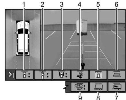
Touch the camera view buttons along the bottom of the infotainment display to access each view (if equipped):
