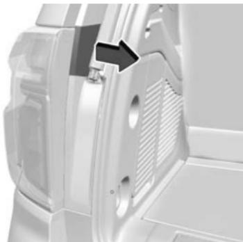
2. Remove the middle trim piece by pulling towards the center of the vehicle to disengage the clips.
