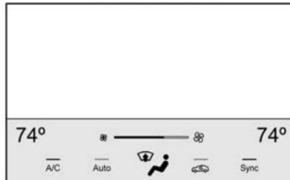
On some models, the climate control status display appears briefly when the center stack climate controls are adjusted.
