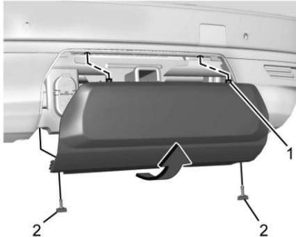
To remove hitch cover, if equipped:
