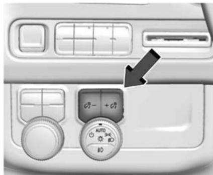
This feature adjusts the brightness of all illuminated controls. The instrument panel illumination control is above the exterior lamp control.
