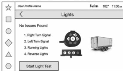
This view will display the names of the trailer connector pins, a graphic of the trailer connector, and a graphic of the back of the trailer.
