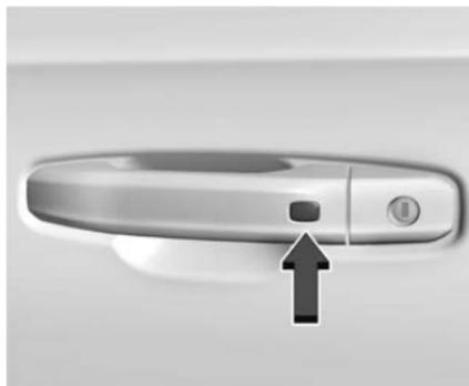
The remote key must be within 1 m (3 ft) of the liftgate or door being opened or locked. Press the button on the door handle to open. See “Keyless Access Operation” in *Remote Key Operation* ⇨ 8.
