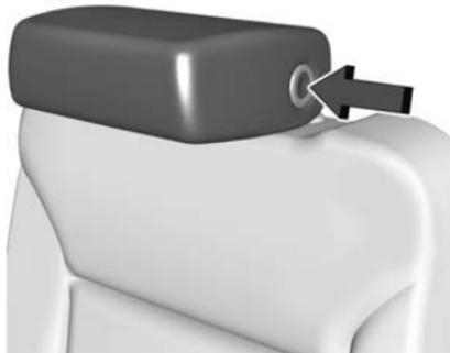
The head restraint will fold forward automatically.
