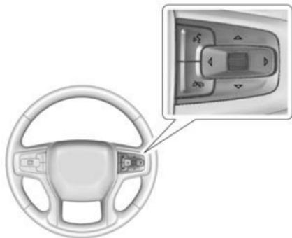
◀ or ▶ : Press to move left or right between the interactive display zones in the instrument cluster. Press the thumbwheel to select.
