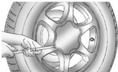
2. If the vehicle has a center cap that covers the wheel fasteners, place the chisel end of the wheel wrench in the slot on the wheel and gently pry the cap out.
