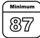
Regular unleaded gasoline meeting ASTM specification D4814 with a posted octane rating (R+M)/2 of 87 or greater is recommended. Do not use gasoline with a posted octane rating of less than 87, as this will result in reduced performance and driveability. If heavy knocking is heard when using gasoline rated at 87 or greater, the engine needs service.
