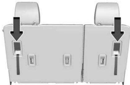
1. Pull up on the lever to release the seatback.
