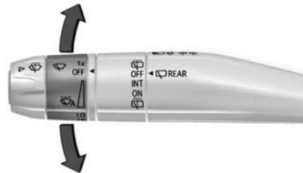
With the ignition on or in accessory mode, move the windshield wiper band to select the wiper speed.
