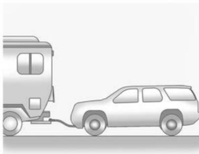
Only dinghy tow four-wheel-drive vehicles with a two speed transfer case that has an N (Neutral) and a 4↓ setting.
