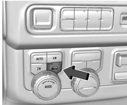
If equipped, select Terrain Mode by pressing the
