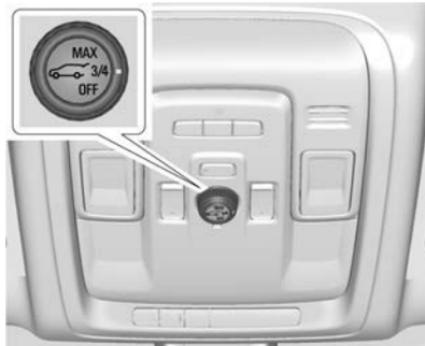
If equipped, the power liftgate switch is on the overhead console. The vehicle must be in P (Park).
