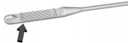
If the oil is below the cross-hatched area at the tip of the dipstick and the engine has been off for at least 15 minutes, add 1 L (1 qt) of the recommended oil and then recheck the level. See “Selecting the Right Engine Oil” later in this section for an explanation of what kind of oil to use. For engine oil crankcase capacity, see *Capacities and Specifications* ⇨ 408.
