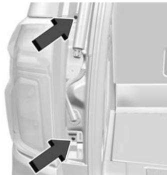
4. Remove the two rear lamp assembly screws.
