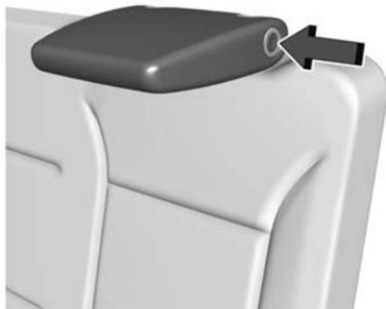
The head restraint will fold forward automatically.
