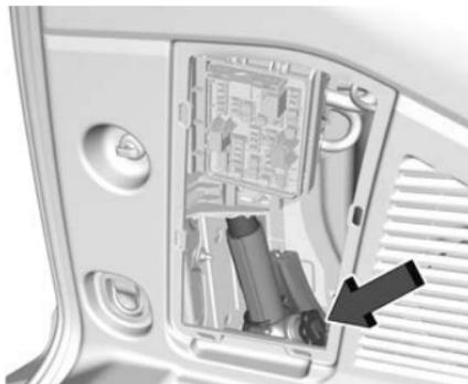
2. Turn the jack knob counterclockwise to release the jack and wheel blocks from the bracket. If equipped, remove the wheel blocks from the jack and place the wheel blocks on both sides of the tire at the opposite corner of the tire being changed. See *If a Tire Goes Flat* ⇨ 371 for more information on the placement of the wheel blocks. Place the jack and wheel blocks near the tire being changed.
