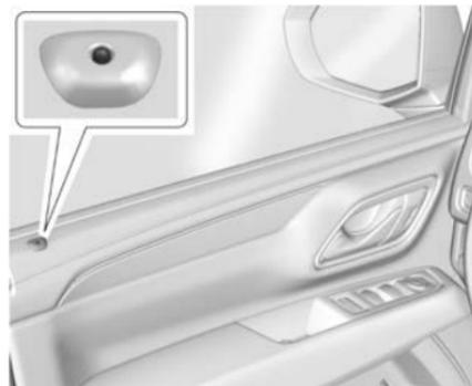
The indicator light, on the driver door near the window, indicates the status of the system. See *Power Door Locks* ⇨ 15
