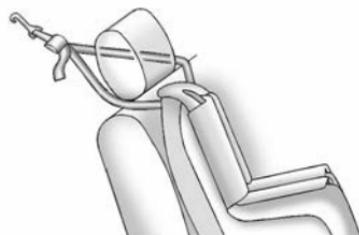
If the position you are using has a fixed or an adjustable head restraint and you are using a dual tether, route the tether around the head restraint.
