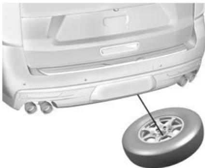
7. Tilt the tire toward the vehicle with some slack in the cable to access the tire/wheel retainer.
