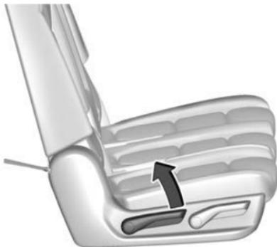
1. Lift the lever on the outboard side of the seat.
