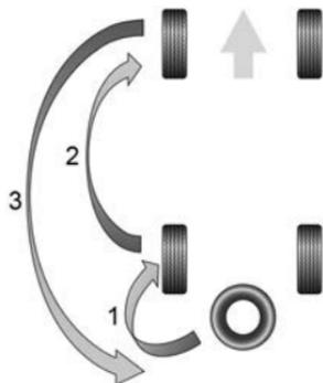
1. Remove the rear tire and replace it with the spare tire by performing all steps in Removing the Flat Tire and Installing the Spare Tire.
