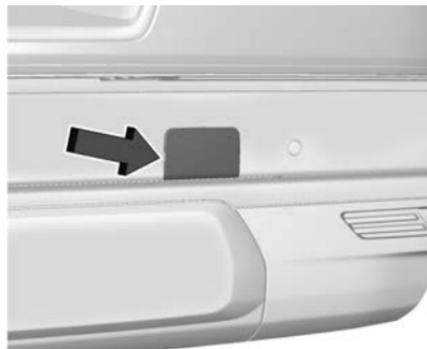
1. Open the hoist shaft access cover (3) on the bumper to access the spare tire lock (6).
