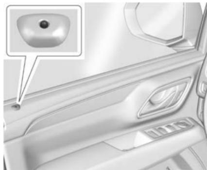
A light on the upper surface of the driver door trim is used to indicate vehicle security status.
