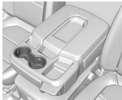
The cupholders are in front of the center console storage area when the armrest is down. See *Center Console Storage* ⇨ 90.
