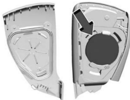
3. Remove the seal by pulling on the tab to access the battery.
