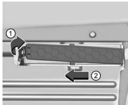
4. Pull the lever (1) on the left side of the filter door and slide left (2), then remove the door. Remove the old filter.
