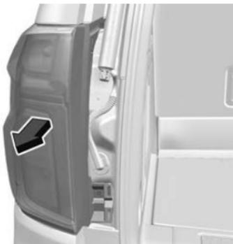
5. Pull the rear lamp assembly rearward to remove it from the vehicle.
