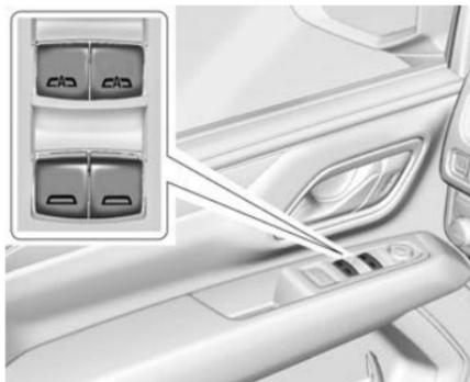
The power windows work when the ignition is on, in accessory mode, or when Retained Accessory Power (RAP) is active. See *Retained Accessory Power (RAP)* ⇨ 212.
