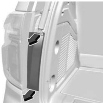
3. Remove the lower taillamp closeout cover from the taillamp assembly by pulling rearward from the top and bottom to disengage the clips.
