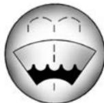
Open the cap with the washer symbol on it. Add washer fluid until the tank is full. See *Engine Compartment Overview* ⇨ 322 for reservoir location.
