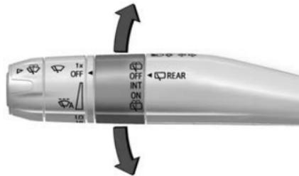
If equipped, turn the windshield wiper band fully upward or downward to spray washer fluid on the rear camera. The wipers will clear the rear camera and either stop or
