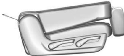
The seatback will fold forward to create a flat load floor.
