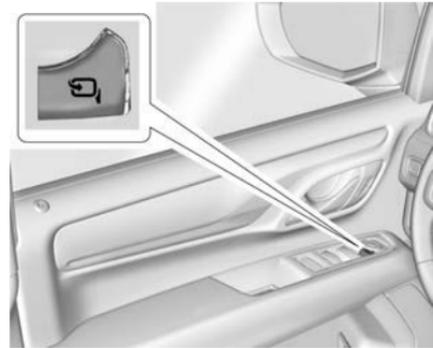
To adjust power folding mirrors, if equipped:
