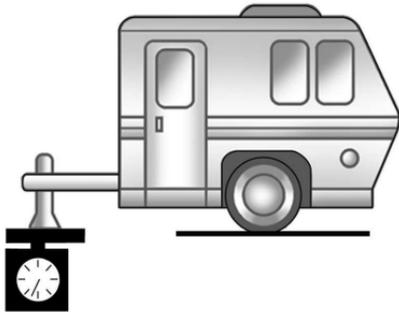
The Maximum Trailer Tongue Weight Rating for a conventional trailer hitch is shown on the Trailing Information Label.
