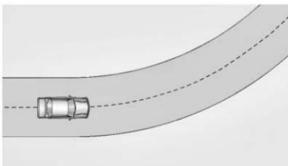
When entering a curve, Super Cruise may not detect the lane markings and may not adjust the steering enough to stay in your lane of travel. When this happens, you will need to steer the vehicle.
