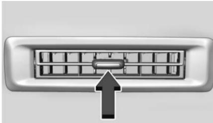
To open a rectangular outlet, move the slider knob and rotate the outlet barrel left to right to change the direction of the air flow and to shut off the air flow.
