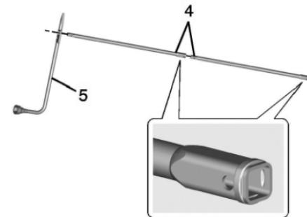
2. Assemble the jack handle extensions (4) and wheel wrench (5), as shown.
