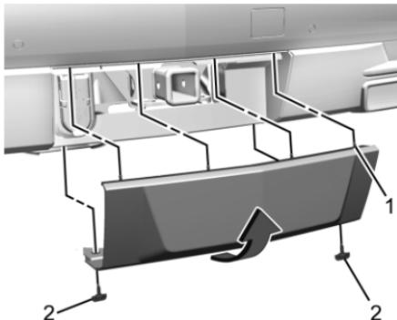
To remove hitch cover, if equipped:
