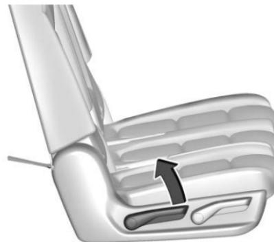
1. Lift the lever on the outboard side of the seat.
