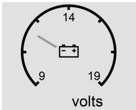
When the ignition is on, the voltmeter gauge indicates the battery voltage.
