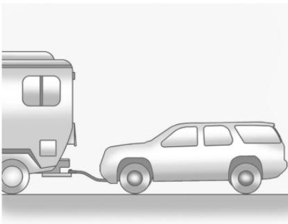
Only dinghy tow four-wheel-drive vehicles with a two speed transfer case that has an N (Neutral) and a 4 $\downarrow$  setting.
