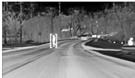
With the Pedestrian Braking system turned on, Night Vision provides a red Head-Up Display (HUD) alert when the system detects that the vehicle is approaching a pedestrian ahead too quickly. In addition, an alert beeps or the Safety Alert Seat pulses, if equipped. See *Front Pedestrian Braking (FPB) System* ▷ 296.
