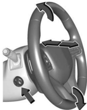
To adjust the power tilt and telescoping steering wheel:
