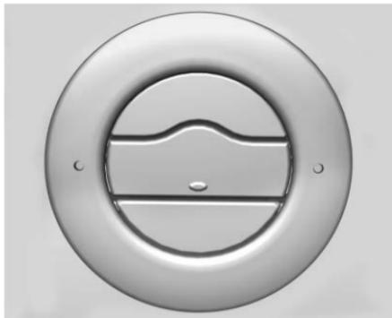
To open a round outlet, press on the center vane bump. Use the center vane to rotate the outlet and change the direction of the airflow. Press on the center vane leading edge to shut off the air flow.
