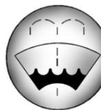
Open the cap with the washer symbol on it. Add washer fluid until the tank is full. See *Engine Compartment Overview* ▷ 346 for reservoir location.
