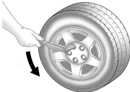
3. Use the wheel wrench to loosen all the wheel nuts. Turn the wheel wrench counterclockwise to loosen the wheel nuts. Do not remove the wheel nuts yet.
