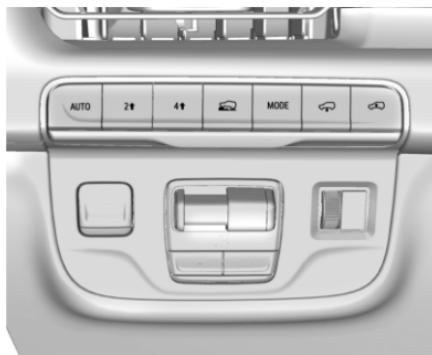
To activate each mode, press the MODE button on the instrument panel to the left of the steering wheel. To activate Terrain mode, press
