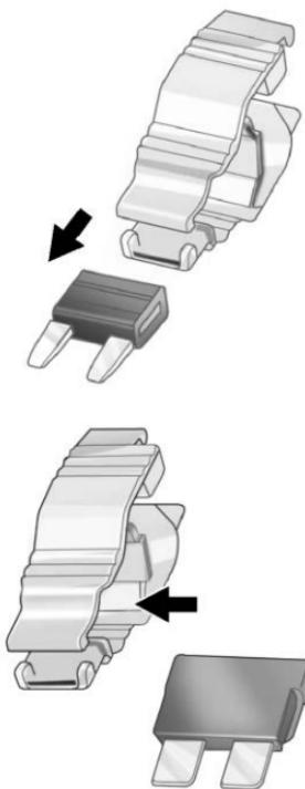
3. Use the fuse puller to remove the fuse from the top or side, as shown above.
