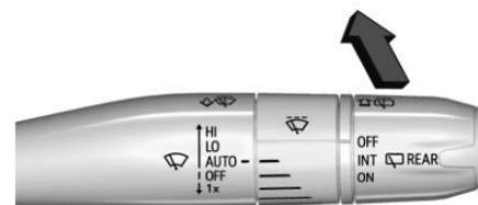
If equipped, push the windshield wiper lever forward to spray washer fluid on the rear camera lens. The lever returns to its starting position when released. See *Rear Camera Mirror* ▷ 32.
