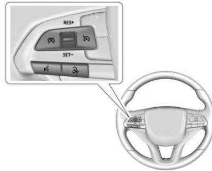
⌚: Press to turn cruise control on or off. The cruise control indicator light ⌚ is lit white on the instrument cluster when cruise control is turned on.
