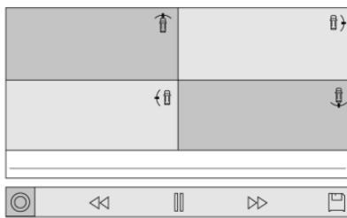
**To Activate:** Touch Video Recorder on the Home Page. Touch the red dot. The red dot will illuminate when the video recorder is on. It will remain on until it has been turned off. Recording will start after exiting the playback screen. Advise other drivers and occupants of the vehicle that video images are being recorded.
