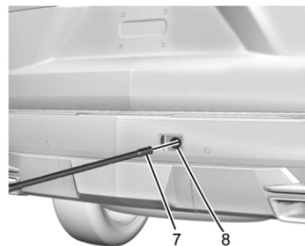
3. Insert the hoist end (open end) of the extension tool (7) through the hoist shaft access hole (8) in the rear bumper until you feel engagement with the hoist assembly (1). Only a minimal amount of the jack handle extension end will be visible.
