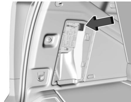
Insert an SD card into the card reader in the trunk. Disable the system from the playback screen before removing the SD card from the reader. Do not remove the card while recording is enabled. This could corrupt the video file and/or the SD card.
