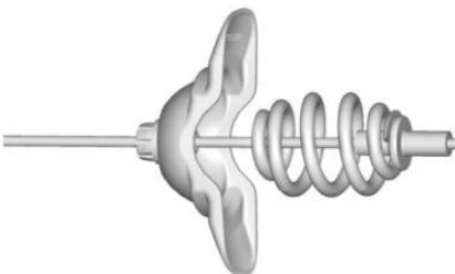
Tilt the retainer and pull it and the cable and spring through the center of the wheel.
