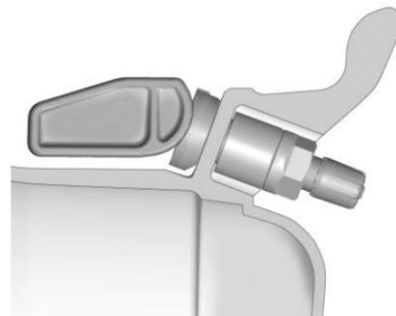
Contact your trailer service center or tire service center to have the pressure sensors installed inside the trailer tires. The technician should insert the sensor stem through the hole in the trailer wheel. When the sensor is correctly positioned, the nut on the sensor stem should
