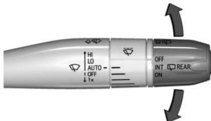
The rear window wiper/washer controls are on the end of the windshield wiper lever.
