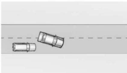
Super Cruise may not detect a vehicle that enters your lane, or may not brake fast enough to avoid a crash. You must manually brake and steer the vehicle.
