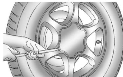
2. If the vehicle has wheel nut caps, loosen them by turning the wheel wrench counterclockwise.
