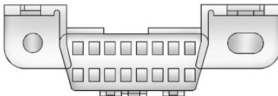
The DLC is under the instrument panel to the left of the steering wheel. Connecting devices that are not used to perform an Emissions Inspection/Maintenance test or to service the vehicle may affect vehicle operation. See *Add-On Electrical Equipment* ▷ 340. See your dealer if assistance is needed.
