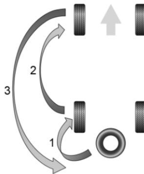
1. Remove the rear tire and replace it with the spare tire by performing all steps in *Removing the Flat Tire and Installing the Spare Tire*.
