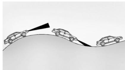
Do not use ACC when driving on steep hills as ACC may not detect a vehicle ahead.
