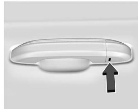
2. Insert the mechanical key into the slot at the bottom of the handle and push upward all the way until the cover frees. Do not pry or pull on the key.
