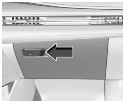
Pull the handle from the side to open the glove box. To close, push the glove box up until it latches. Use the mechanical key in the remote key to lock or unlock. See *Keys* ▷ 6.
