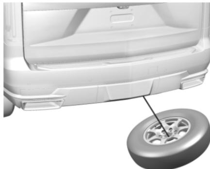
6. Tilt the spare tire toward the vehicle with some slack in the hoist cable (11) to access the tire/wheel retainer (10).
