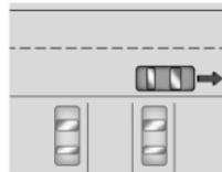
After completely passing an eligible parking spot, a beep sounds and a red stop symbol is displayed in the driver information center. Generally, APA selects the nearest empty parking spot behind the vehicle, but under some conditions may select a space that is further back. Slow down and bring the vehicle to a complete stop to begin.
