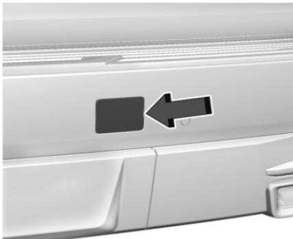
1. Open the spare tire lock cover on the bumper and use the mechanical key to remove the spare tire lock (6). To remove the spare tire lock, insert the mechanical key, turn, and pull straight out.
