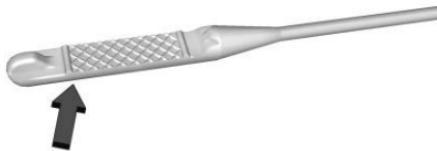
If the oil is below the cross-hatched area at the tip of the dipstick and the engine has been off for at least 15 minutes, add 1 L (1 qt) of the recommended oil and then recheck the level. See "Selecting the Right Engine Oil" later in this section for an explanation of what kind of oil to use. For engine oil crankcase capacity, see *Capacities and Specifications* ▷ 436.
