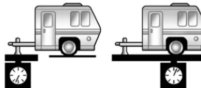
The trailer tongue weight (1) should be 10–15% of the total loaded trailer weight (2). Some specific trailer types, such as boat trailers, fall
