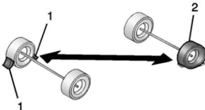
1. If equipped, place wheel blocks (1), as shown, to prevent the vehicle from moving.
