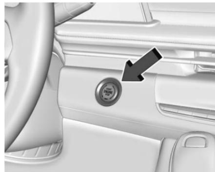
Vehicles equipped with Keyless Access have pushbutton starting.
