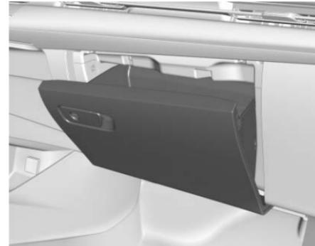
1. Open the glove box door completely.
