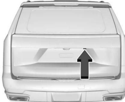
Press the button above the license plate to open the liftglass, or press
