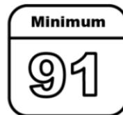
Premium unleaded gasoline meeting ASTM specification D4814 with a posted octane rating (R+M)/2 of 91 or greater is recommended. If unavailable, unleaded gasoline with a posted octane rating of 87 may be used, but will result
