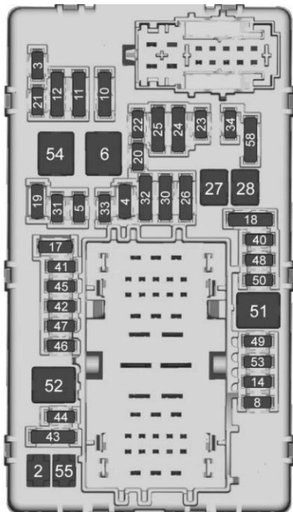
There are relays on the back of the fuse block. To access, press the tabs and remove the fuse block.
