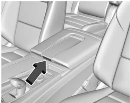
Press the button and lift to open. There is an auxiliary jack, USB ports, an accessory power outlet, a tote compartment, and a device holder inside.
