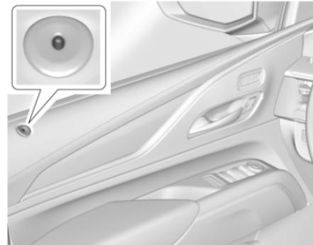
A light on the upper surface of the driver's door trim is used to indicate vehicle security status.
