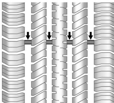
Treadwear indicators are one way to tell when it is time for new tires. Treadwear indicators appear when the tires have only 1.6 mm (1/16 in) or less of tread remaining. See *Tire Inspection* ▷ 390 and *Tire Rotation* ▷ 390.
