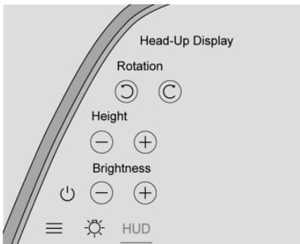
The HUD control is on a touchscreen to the left of the instrument cluster. HUD controls are also available on the infotainment screen. See *Settings* ▷ 186.
