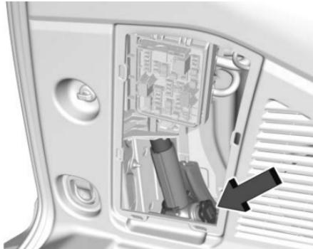
2. Turn the jack knob counterclockwise to release the jack and wheel blocks from the bracket. If equipped, remove the wheel blocks from the jack and place the wheel blocks on both sides of the tire at the opposite corner of the tire being changed. See *If a Tire Goes Flat* ▷ 395 for more information on the placement of the wheel blocks. Place the jack and wheel blocks near the tire being changed.
