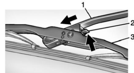
2. Push the release lever (2) to disengage the hook and push the wiper arm (1) out of the blade assembly (3).
