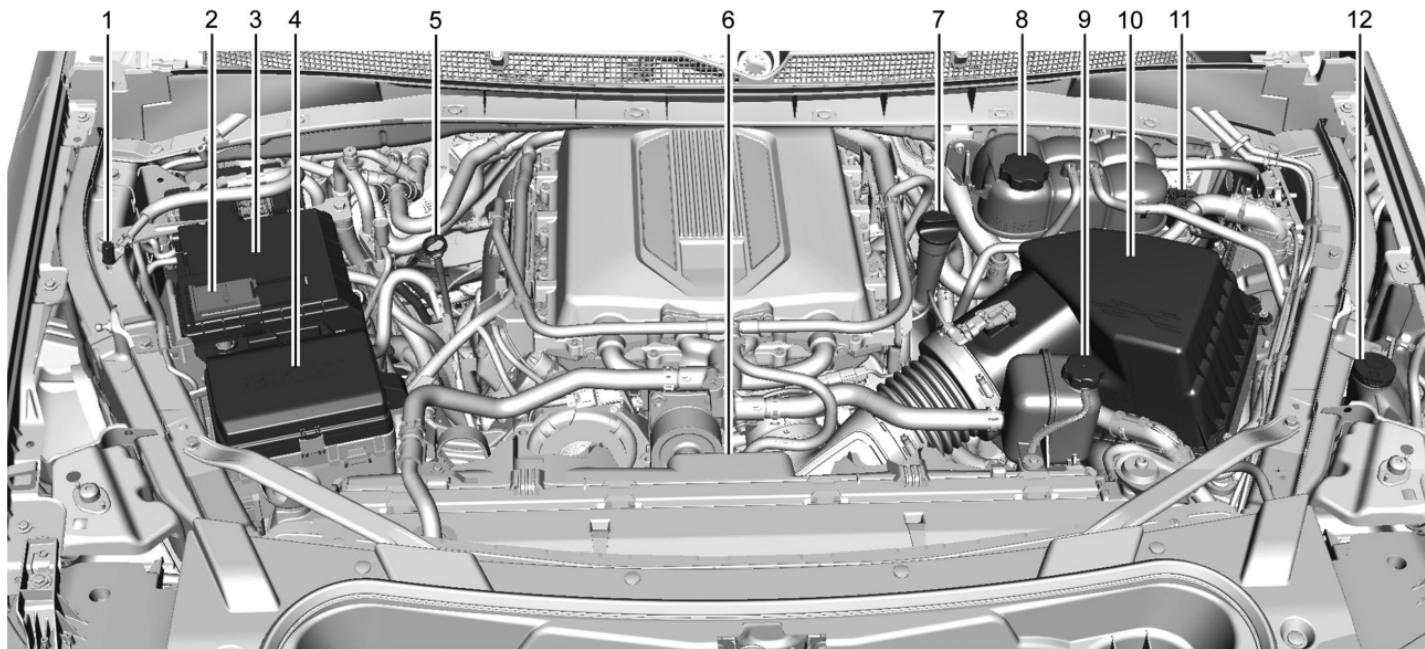
6.2L V8 Supercharged Engine (LT4)
