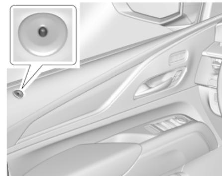
The indicator light, on the driver door near the window, indicates the status of the system. See **Power Door Locks ▷ 17**
