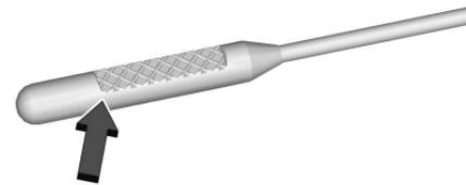
If the oil is below the cross-hatched area at the tip of the dipstick and the engine has been off for at least 15 minutes, add 1 L (1 qt) of the recommended oil and then recheck the level. See “Selecting the Right Engine Oil” later in this section for an explanation of what kind of oil to use. For engine oil crankcase capacity, see *Capacities and Specifications* ▷ 306.
