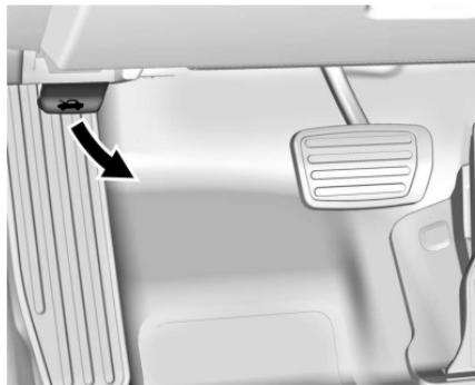
1. Pull the hood release lever with the
