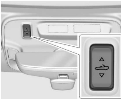
5. Press and hold the bottom of the switch. The windows will automatically lower.
