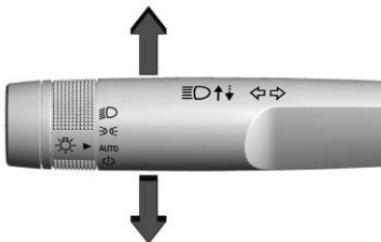
Move the lever all the way up or down to signal a turn.
