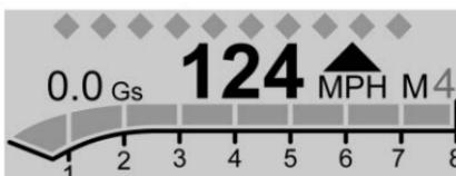
**Performance View** : If equipped, displays digital speed, indicators from speed view, rpm reading, transmission positions, gear shift indicator, Shift Timing Light Position, and lateral acceleration (G) indicators.
