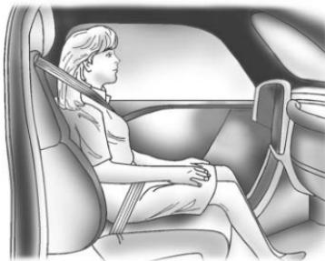
If a person of adult size is sitting in the front outboard passenger seat, but the OFF indicator is lit, it could be because that person is not sitting properly in the seat or that the child restraint locking feature is engaged. Use the following steps to allow
