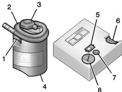
1. Sealant Canister Inlet Valve
