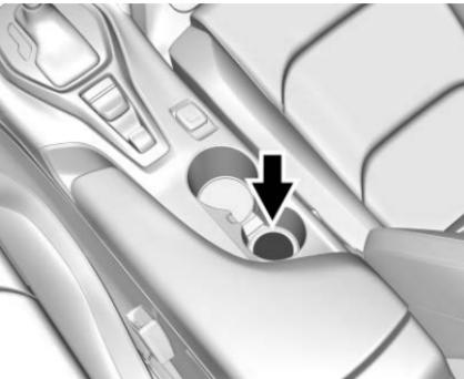
5. Replace the recognized remote keys with a new remote key. Place the new remote key in the rear cupholder in the center console.
