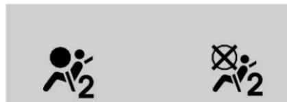
The words ON and OFF, or the symbols for on and off, will be visible during the system check. When the system check is complete, either the word ON or OFF, or the symbol for on or off will be visible. See *Passenger Airbag Status Indicator* ▷ 91.
