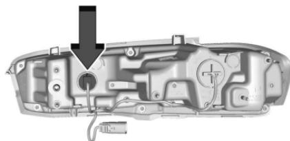
For the base and the uplevel taillamp assembly, only the back-up bulb is replaceable. Removal of the taillamp assembly is not necessary to change this bulb.
