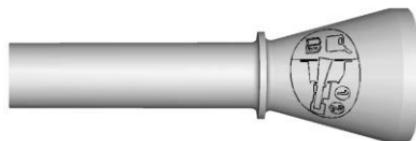
1. Locate the capless funnel adapter from under the carpet in the trunk.
