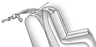
If the child restraint has a dual tether, route the tether over the seatback.
