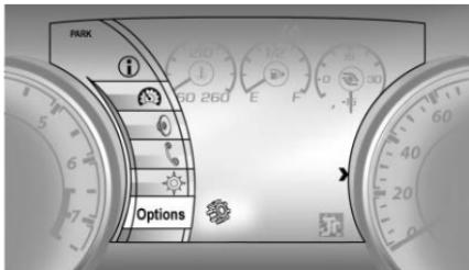
1. Using the buttons on the right side of the steering wheel, press ▲ to open the top level DIC menu. Use ▽ to scroll down to Options and press SEL.
