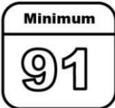
Premium unleaded gasoline meeting ASTM specification D4814 with a posted octane rating (R+M)/2 of 91 or greater is required. The use of the correct fuel is an important part of the proper maintenance of the vehicle and a condition of the vehicle warranty. If heavy knocking is heard when using gasoline rated at 91 or greater, the engine needs service.
