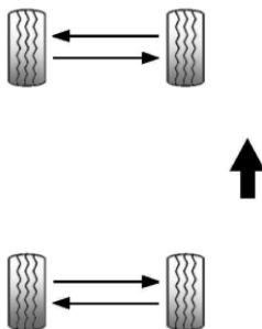
Use this rotation pattern if the vehicle has different size tires on the front and rear.
