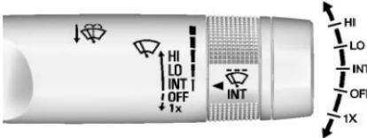
The windshield wiper/washer lever is on the right side of the steering column. With the ignition on or in accessory mode, move the windshield wiper lever to select the wiper speed.
