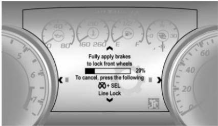
6. Press the brake pedal firmly to move the bar graph to 100%.
