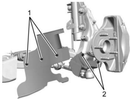
8. Install the small splash shields with two screws (2) per corner. Torque to  $9\text{ N}\cdot\text{m}$  (80 lb inch).
