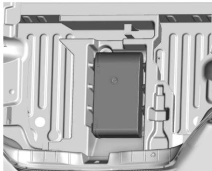
3. Remove the tire sealant and compressor kit bag from the storage foam.
