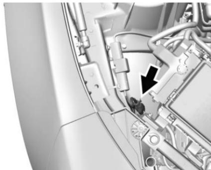
The electrical cord is on the passenger side of the engine compartment, next to the engine compartment fuse block.
