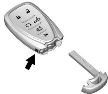
1. Press the button on the side of the remote key and pull the key out. Never pull the key out without pressing the button.
