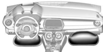
The driver knee airbag is below the steering column. The front outboard passenger knee airbag is below the glove box.
