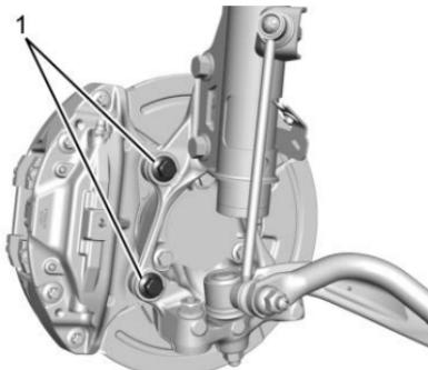
12. Apply liquid thread adhesive to the caliper bolts (GM Part No. 9985399 – Loctite 272 – Goodwrench 12345493). Install the calipers with two screws (1) per corner. Torque the caliper bolts to  $200\text{ N}\cdot\text{m}$  (148 lb ft).
