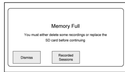
If there is no available space on the SD card, a message displays. Delete or transfer recordings on the SD card or use another SD card with free space.
