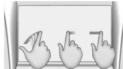
Fling or swipe is used to scroll through a list, pan the map, or change page views. Do this by placing a finger on the display then moving it rapidly up and down or right and left.
