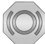
The brake/clutch master cylinder reservoir is filled with GM approved DOT 4 brake fluid as indicated on the reservoir cap. See *Engine Compartment Overview* ▷ 229 for the location of the reservoir.
