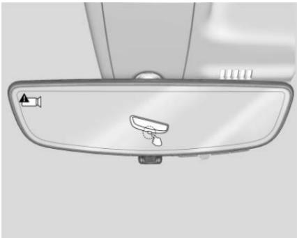
See your dealer for service if a blue screen and
