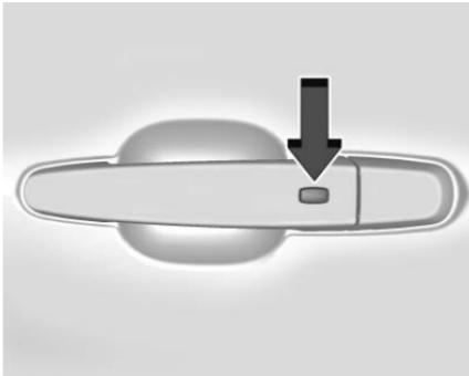
The remote key must be within 1 m (3 ft) of the trunk or door being opened. Press the button on the door handle to open. See "Keyless Access Operation" in *Remote Key Operation* ▷ 7.
