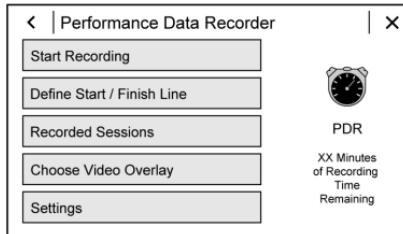
If the system is unable to begin recording, the Start Recording button is grayed out.
