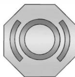
The brake/hydraulic clutch fluid reservoir cap has this symbol on it. See *Engine Compartment Overview* ▷ 229 for reservoir location. The common hydraulic clutch and brake master cylinder fluid reservoir is filled with brake fluid as indicated on the reservoir cap. See *Brake Fluid* ▷ 244 for brake fluid to use.
