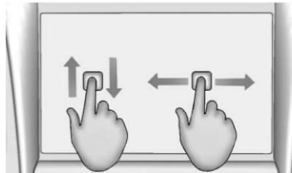
Drag is used to move applications on the Home Page, or to pan the map. To drag the item, it must be held and moved along the display to the new location. This can be done up, down, right, or left. This feature is only available when vehicle is parked and not in motion.
