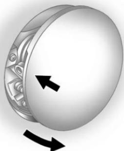
To open the fuel door, push and release the rearward center edge of the door.
