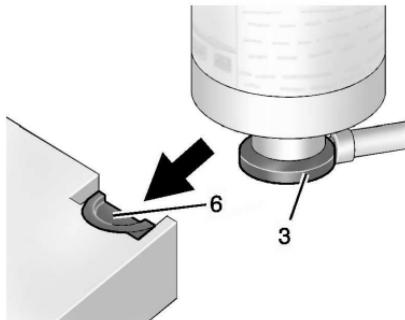
5. Slide the base of the tire sealant canister (3) into the slot on the top of the compressor (6) to hold it upright. Make sure the tire valve stem is positioned close to the ground so the hose will reach it.
