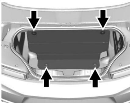
The trunk partition can be attached or detached to upper trunk brackets. With the convertible top up, the trunk partition can be unsnapped and laid flat.
