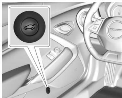
From inside the vehicle, press
