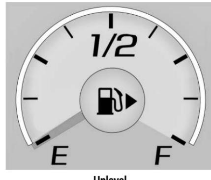
When the ignition is on, the fuel gauge indicates the approximate amount of fuel left in the tank.
