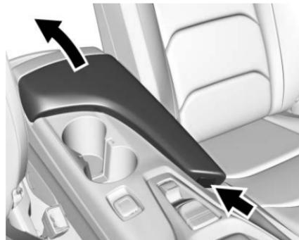
Press to open. If equipped, there are two USB ports and an auxiliary jack inside. See *USB Port* ▷ 121 and *Auxiliary Jack* ▷ 123.
