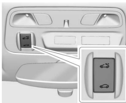
If equipped, the sunroof only operates when the ignition is on or in accessory mode, or when Retained Accessory Power (RAP) is active. See *Retained Accessory Power (RAP)*  $\Rightarrow$  194.
