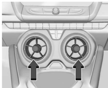
Use the air outlets in the center and on the side of the instrument panel to direct the airflow. Turn the center knobs on the air outlets clockwise or counterclockwise to open or close off the airflow.
