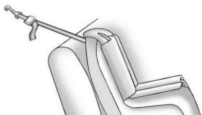
If the child restraint has a single tether, route the tether over the seatback.
