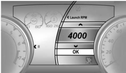
8. Adjust the desired RPM using △ or ▽:
