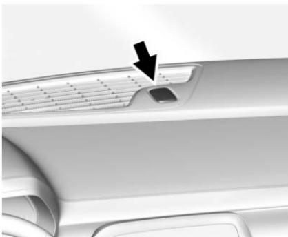
The security light, on the instrument panel near the windshield, indicates the status of the system:
