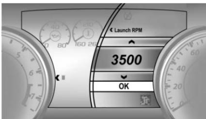
9. Press SEL to confirm the desired RPM.
