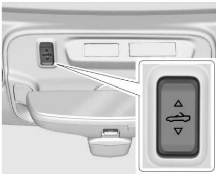
6. Press and hold the top of the switch. The windows will automatically lower.
