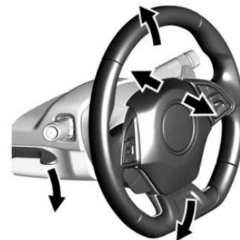
To adjust the tilt and telescoping steering wheel:
