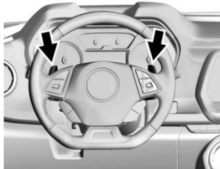
The system is activated and deactivated by pressing either of the paddles marked REV MATCH on the steering wheel. The system must be activated with each new ignition cycle.
