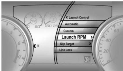
6. Scroll down to Launch RPM using ▽.
