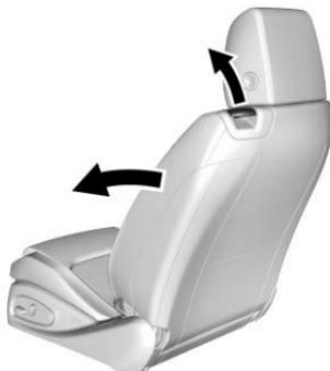
To access the rear seats, pull up on the latch on the top of the driver or front passenger seatback. Fold the seatback forward.
