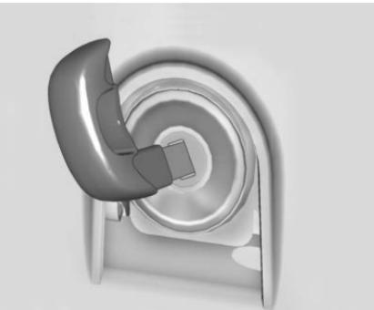
5. Remove any additional items attached to the key — such as keys, rings, or tags — then fully insert the key into the manual release.
