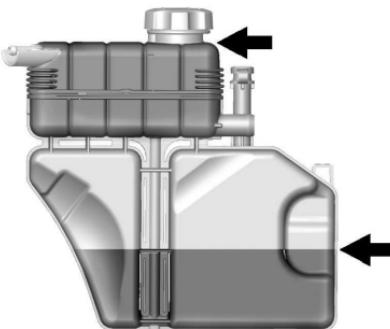
3. Fill the surge tank top chamber with the proper mixture to the bottom of the fill neck. The top chamber needs to be completely full. Fill the surge tank bottom chamber through the service port to approximately half.
