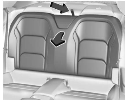
Pull the loop on the center of the rear seat back. The rear seat back will fold down.
