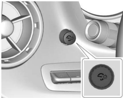
This feature adjusts the brightness of all illuminated controls. The knob for this feature is on the left side of the instrument panel.
