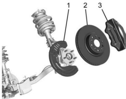
3. Remove the calipers (3) from the knuckle.
