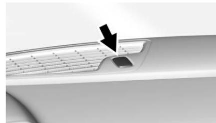
The vehicle has a light sensor on the top of the instrument panel. Do not cover this sensor, otherwise the system will come on whenever the ignition is on.
