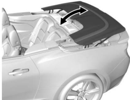
1. On each side of the tonneau cover, lift and pivot rearward into the fully open position. Hold the front and rear of the tonneau cover at the same time.
