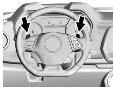
Tap Shift allows you to manually control the automatic transmission. To use Tap Shift, the shift lever must be in DSC mode. Vehicles with this feature have indicators on
