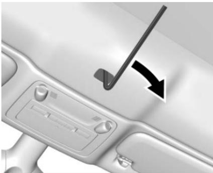
3. Lock the front of the convertible top to the frame by popping out the small cover, inserting a hex wrench, and turning clockwise until it stops.
