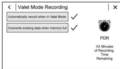
**Valet Mode Recording :** Allows recording preferences to be selected. It is recommended that a blank SD card be used. Available choices are:
