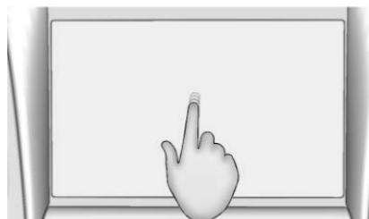
Nudge is used to move items a short distance on a list or a map. To nudge, hold and move the selected item up or down to a new location.
