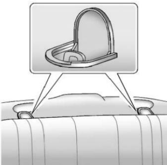
On coupe models, the top tether anchors are on the rear seatback filler panel.
