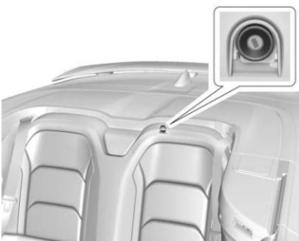
2. Locate the manual release beside the rear seat cushion on the driver side.
